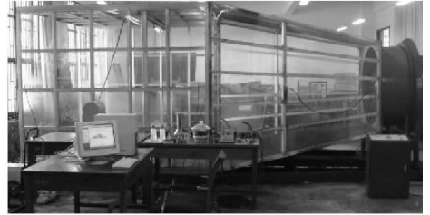
图 2 风流-雾滴-尘粒三相介质耦合作用实验装置 Fig. 2 Airflow-droplet-dust particle three-phase medium coupling device
