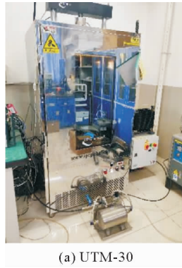
Fig. 2 Four-point bending fatigue test device
